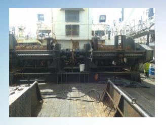
The original electric fishing winch (Siemens, Brusselle, 1983) of RV Oca Balda, was changed in 1997 by hydraulic one of local manufacturing. But it has never worked properly and limited the fishing activities. So we decided to replace the hydraulic winch with a new electric one with today's technology.
