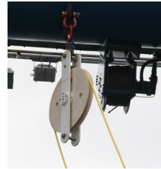
Portable clean CTD block. Sheave made of Nylotron.
