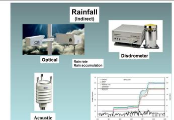
Indirect methods for measuring precipitation. Optical (most common for ships). Plot shows comparisons for different sensors and different locations with ship relative wind speed plotted along the bottom. All sensors capture the various rain events, but with differing degrees of accuracy.
