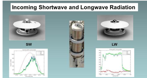
SW (Pyranometer) broadband solar radiance on a planar surface LW (Pyrgeometer) atmospheric infra-red radiation. Good quality radiometers are not cheap but very important to understanding the energy budget. Plots show comparisons between ship (SCS) and Flux Standard (PSD) sensors along with modeled clear sky calculation for incoming SW and downwelling LW radiation.
