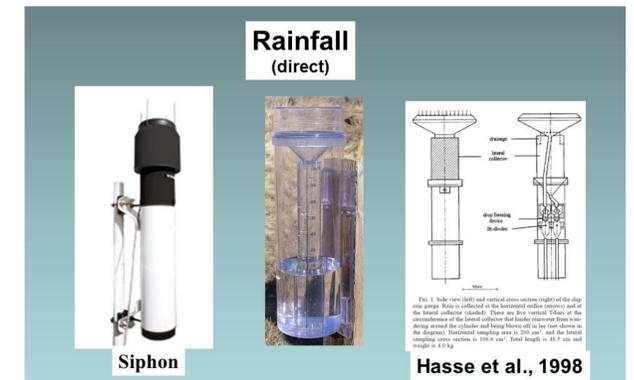
From left to right siphon gauge (common ship sensor), standard land precipitation gauge, and research proto-type gauge designed to minimize wind effects.
