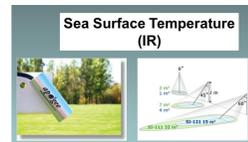
Indirect measurement using IR sensor. Total surface area viewed dependent on tilt angle of sensor.
