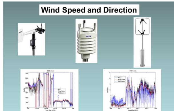
Prop-vane anemometer, 2-D sonic anemometer, 3-D sonic anemometer
