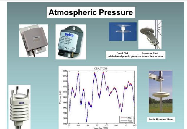
Pressure sensors are similar with varying response times and accuracies depending on your need. For shipboard use it is critical to have a dynamic pressure port connected to the sensor to reduce the dynamic wind effects (Bernoulli Effect). This pressure port should be located in a place on the ship least affected by flow around the ship's structure. Note: The actual pressure is measured at the height of the sensor and not the pressure port. The plot is a comparison of 2 different sensors.
