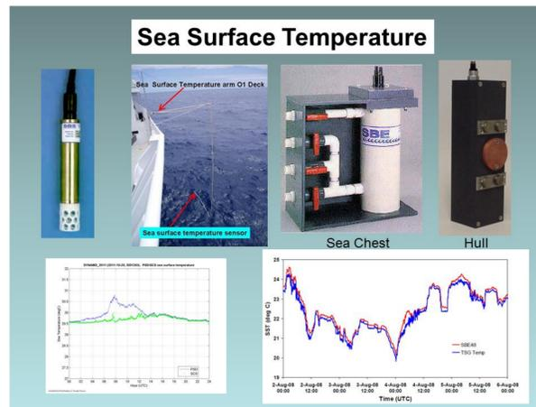
Sensors from left to right: temperature profiling sensor typically used with CTD, "Seasnake" floating thermistor, ship intake, hull mounted. Left plot shows comparison between "Seasnake" (blue) and ship intake sensor (green) with warming from the sun of the "Seasnake". Right plot is comparison of ship intake (blue) and hull (red) sensors showing dampening and delay of hull mounted temperature sensor.
