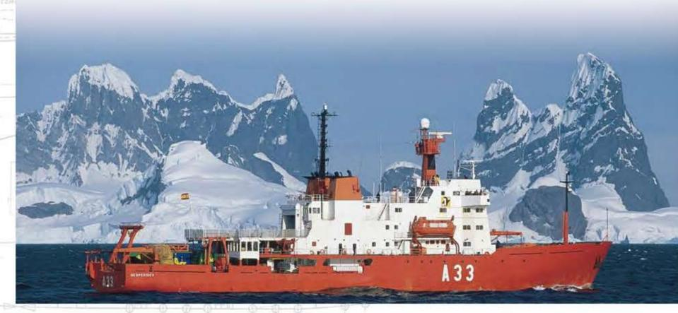
RV García del Cid: multipurpose ship of 37 m overall length, built in 1979. It is therefore the first ship of the CSIC and has developed over the years all types of works in oceanography. It was adapted from a former fishing boat design to a multipurpose RV in late 80's , including a stern gantry, cable
